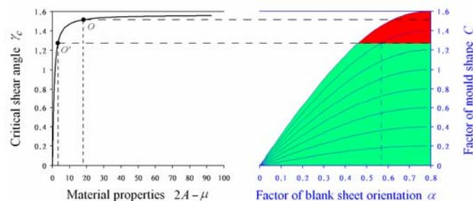
Fig. 6. Illustration of material's formability during stamping
