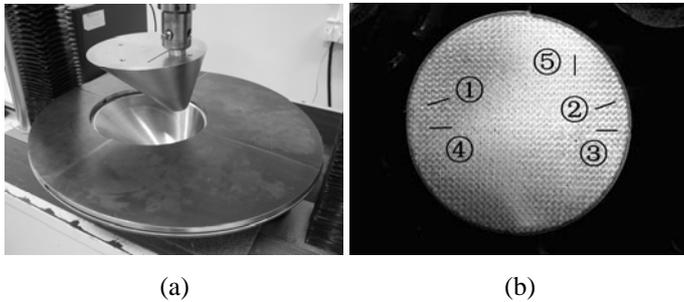
Fig. 1. Stamping set-up: (a) equipment; (b) sample orientation
