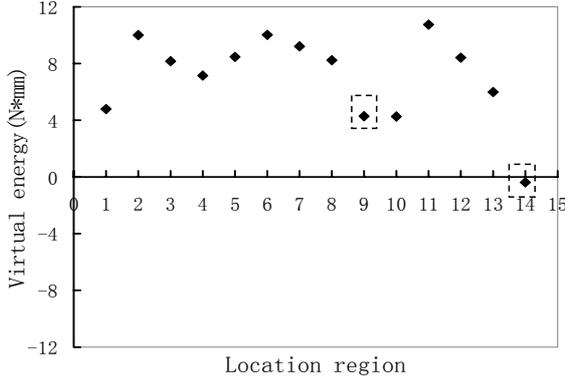
Fig. 4. Virtual wrinkling energies at different locations
