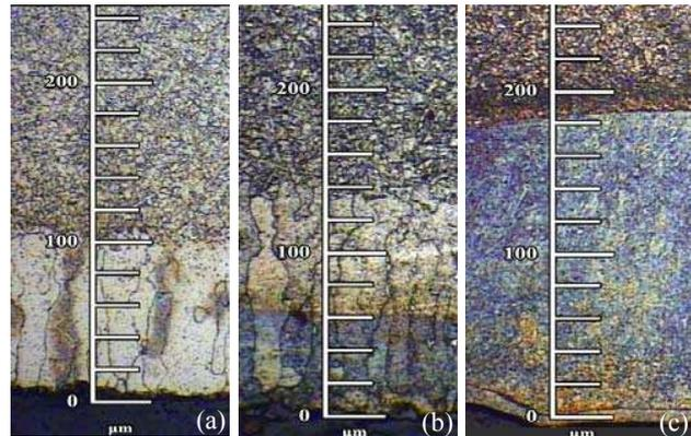
Fig. 2 Through surface micrographs of H13 tool steel laser treated specimens for (a) sample 1; (b) sample 3; and (c) sample 4.
