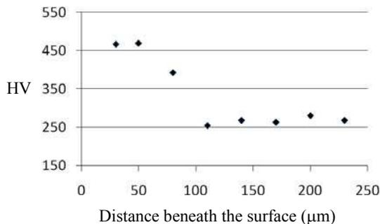
Fig. 5 Average Vickers hardness (HV) measurements taken at set distances below the surface for sample 17.
