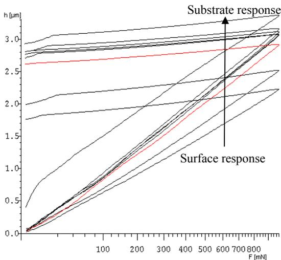
Fig. 1 Stress relief plots for a depth limited micro-hardness setting of 1 N.
