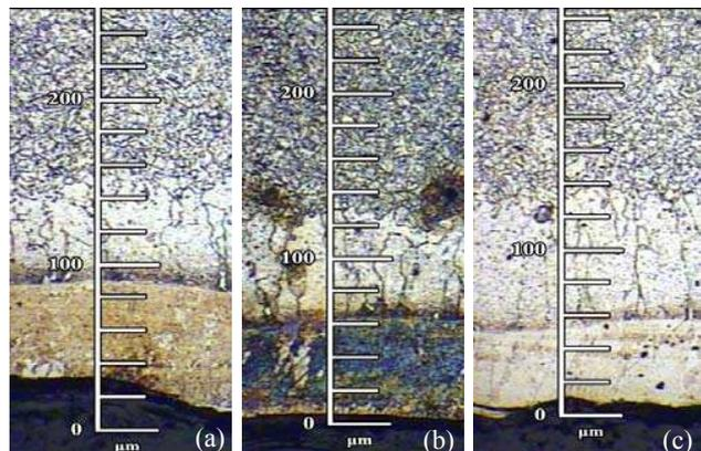
Fig. 3 Through surface micrographs of H13 tool steel laser treated specimens for (a) sample 13; (b) sample 14; and (c) sample 17.
