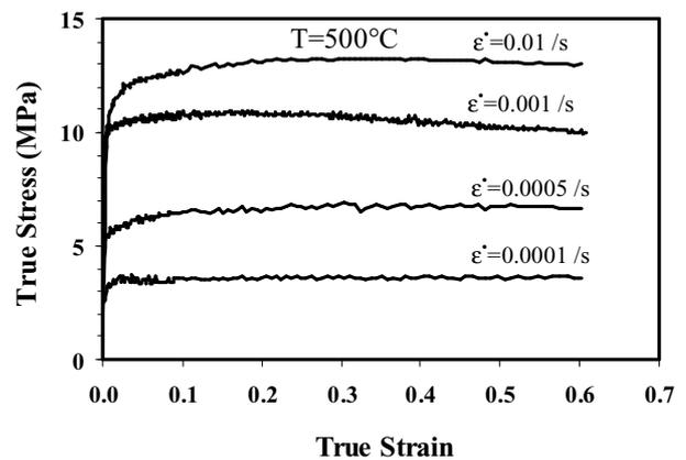
Fig. 3. The true stress-true strain curves at 500°C
