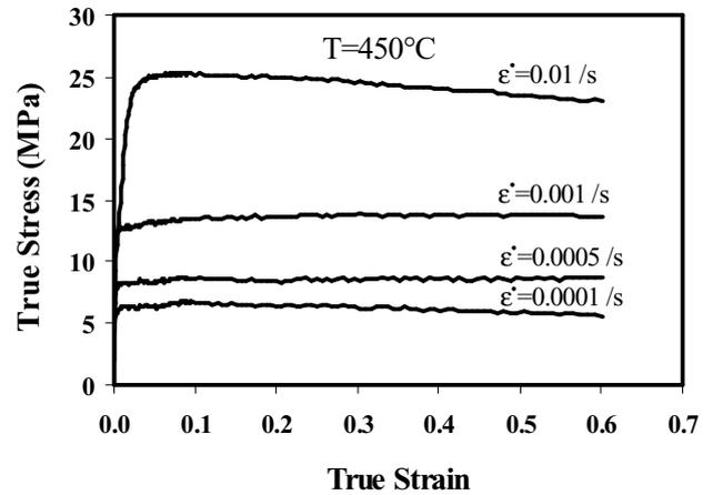
Fig. 2. The true stress-true strain curves at 450°C
