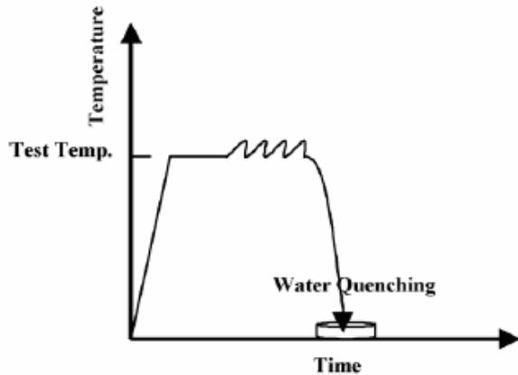
Fig. 1. The schematic representation of the applied thermo-mechanical cycle
