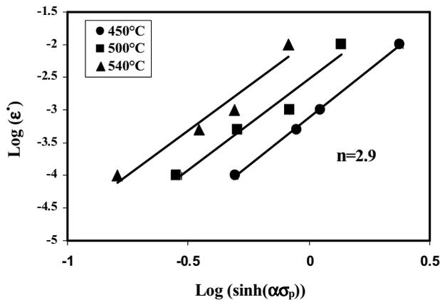
Fig. 6. The variation of strain rate with maximum stress ( $\alpha=0.08$ )
