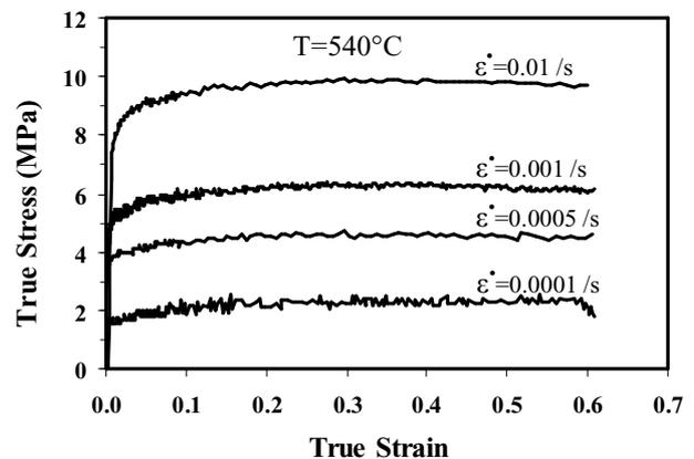
Fig. 4. The true stress-true strain curves at 540°C
