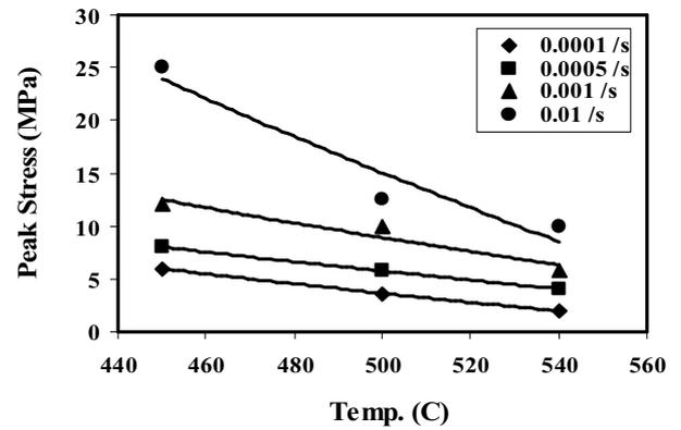
Fig. 5. The variation of maximum stress as a function of temperature
