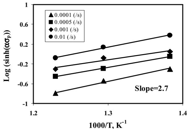
Fig. 7. The variation of maximum stress with temperature ( $\alpha=0.08$ )
