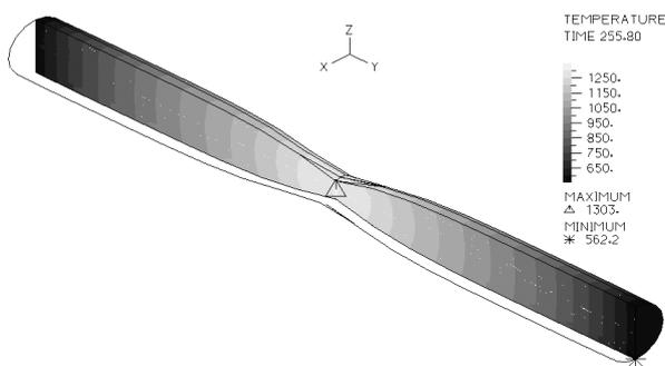
Fig. 5. Distribution of temperature on the surface and inside the sample for the tension test at 1300°C
