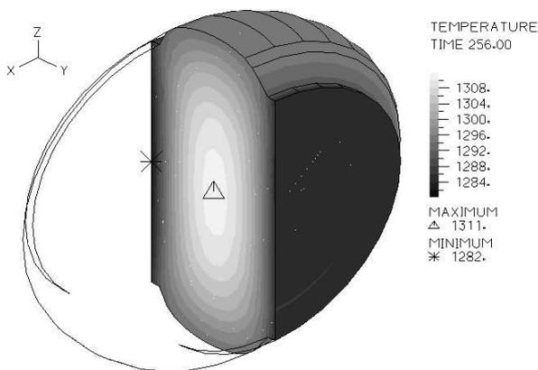
Fig. 3. Distribution of temperature on the surface and inside the sample for the compression test at 1300°C
