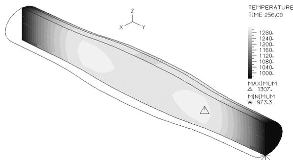
Fig. 4. Distribution of temperature on the surface and inside the sample for the L-Sico test at 1300°C
