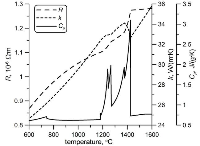
Fig. 2. The thermo-physical properties of M2 tool steel calculated using JMatPro software; electrical resistivity  $R$ , thermal conductivity  $k$ , specific heat  $C_p$
