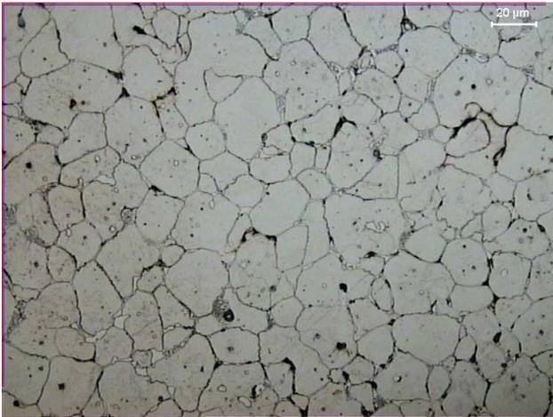
Fig. 6. Optical micrograph of M2 steel heated to 1250°C and next quenched (zero minute holding)
