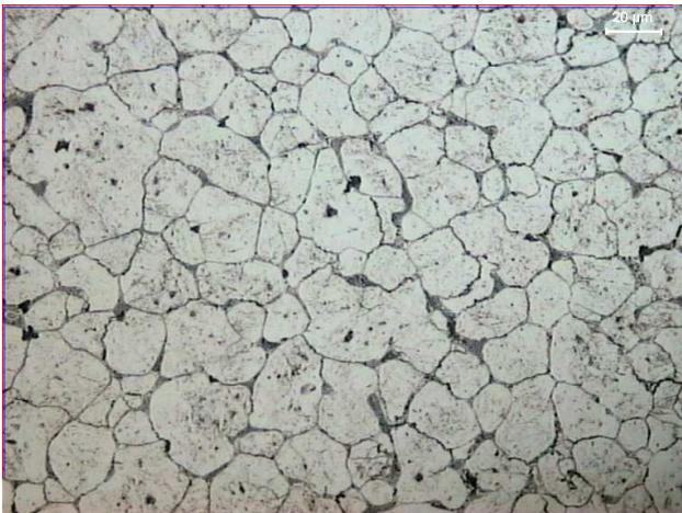
Fig. 7. Optical micrograph of M2 steel heated to 1300°C and next quenched (zero minute holding)
