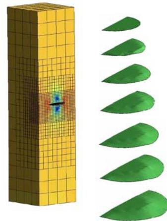
Fig. 3. Example of a 3D crack growth in mixed mode
