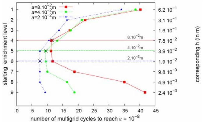
Fig. 2. Link between the finest enriched level and the rate of convergence for a given crack length
