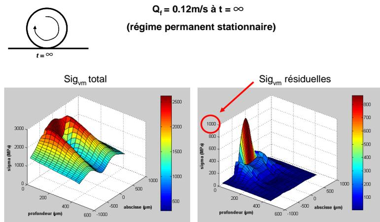
Fig. 3. Von Mises stress under loading (left) and after unloading (right) for a stationary sphere on flat contact under steady-state regime.
