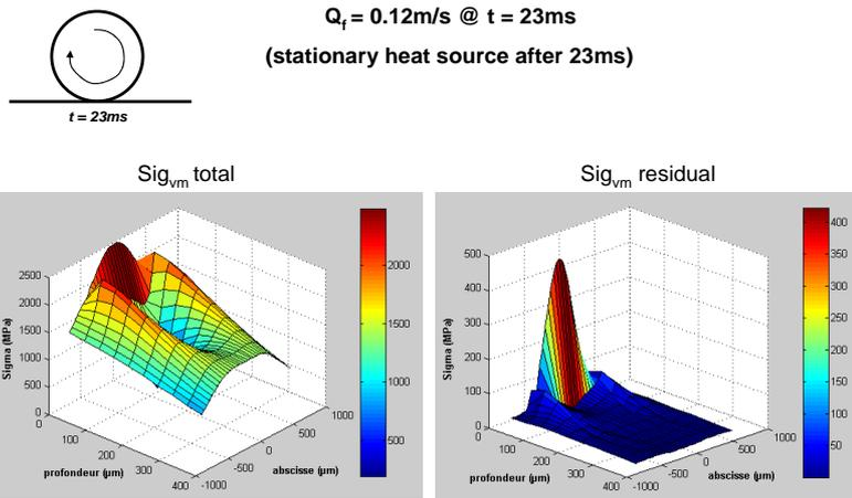
Fig. 2. Von Mises stress under loading (left) and after unloading (right) 23 ms after the beginning of the thermo-mechanical loading for a stationary circular point contact.
