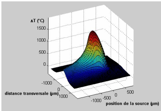
Fig. 5. Surface temperature rise after  $23\text{ ms}$ , for Fig. 4.
