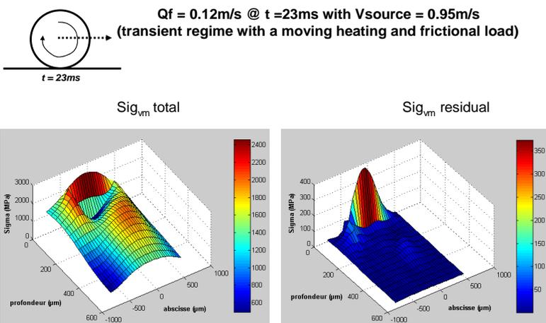
Fig. 4. Von Mises stress under loading (left) and after unloading (right) 23 ms after the beginning of the load/source movement (circular point contact).
