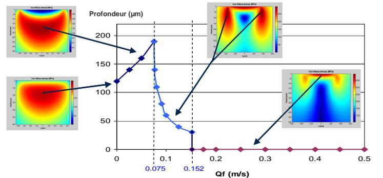
Fig. 1. Depth where the von Mises stress at the onset of yielding is found maximum, versus the heat factor  $Q_f = \mu f \cdot \beta \cdot \Delta U$  (stationary circular point contact).
