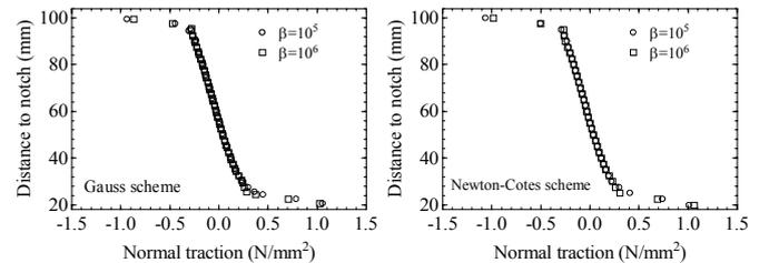
Fig. 5. Effect of integration scheme on traction profiles
