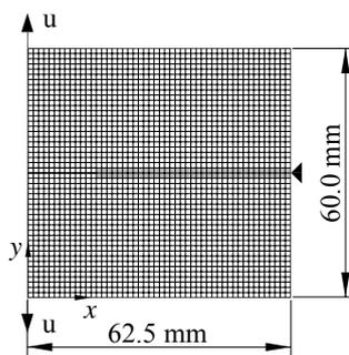
Fig. 6. Geometry of compact test specimen
