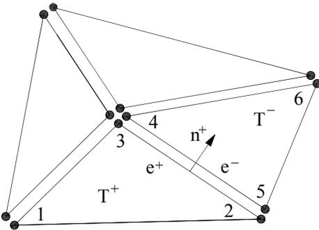
Fig. 2. Discontinuous Galerkin mesh
