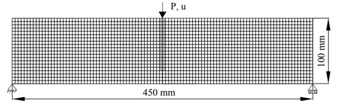
Fig. 4. Geometry of 3-point bending beam
