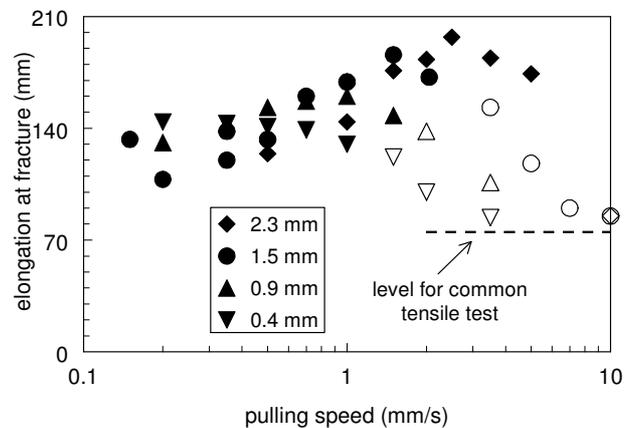
Fig. 6. Elongation at fracture plotted as a function of pulling speed with the depth setting as parameter.
