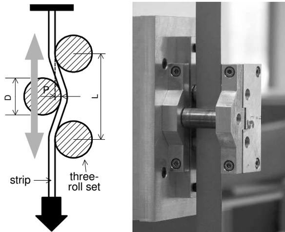
Fig. 2. Left: schematic representation of the test; right: picture of the roll set.
