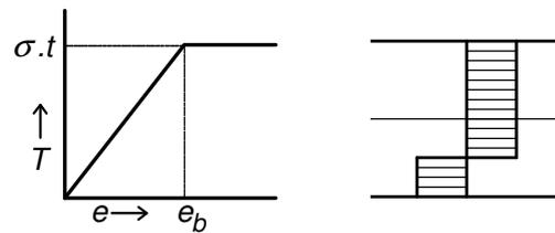
Fig 1. Left: Graphic presentation of equation (1) for a situation of constant bending radius  $R$ ;  $e_b = t/2R$ . Right: stress distribution for the case  $e = e_b/2$ .
