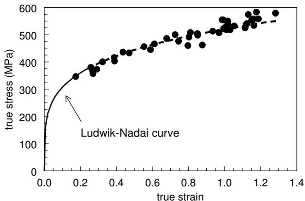
Fig. 7. Hardening curve constructed from the tested specimens.
