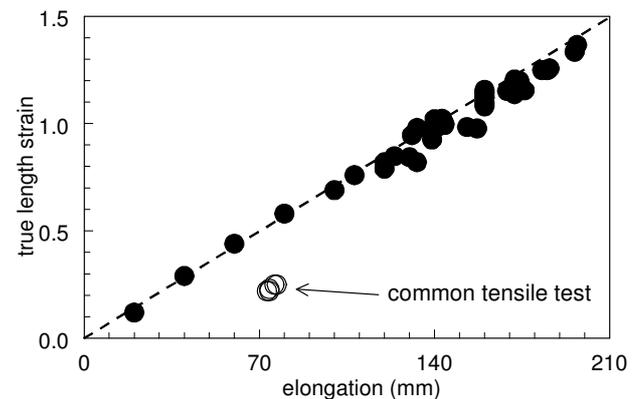
Fig. 3. Relation between measured uniform strain (true strain) and total elongation of the specimen.
