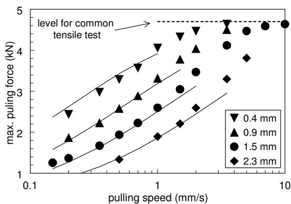
Fig. 5. Maximum pulling force plotted as a function of pulling speed with the depth setting as parameter.
