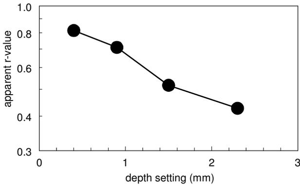
Fig. 4. Ratio between width strain and thickness strain plotted as a function of depth setting.
