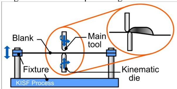
Fig. 1: Theoretical setup for kinematic ISF
