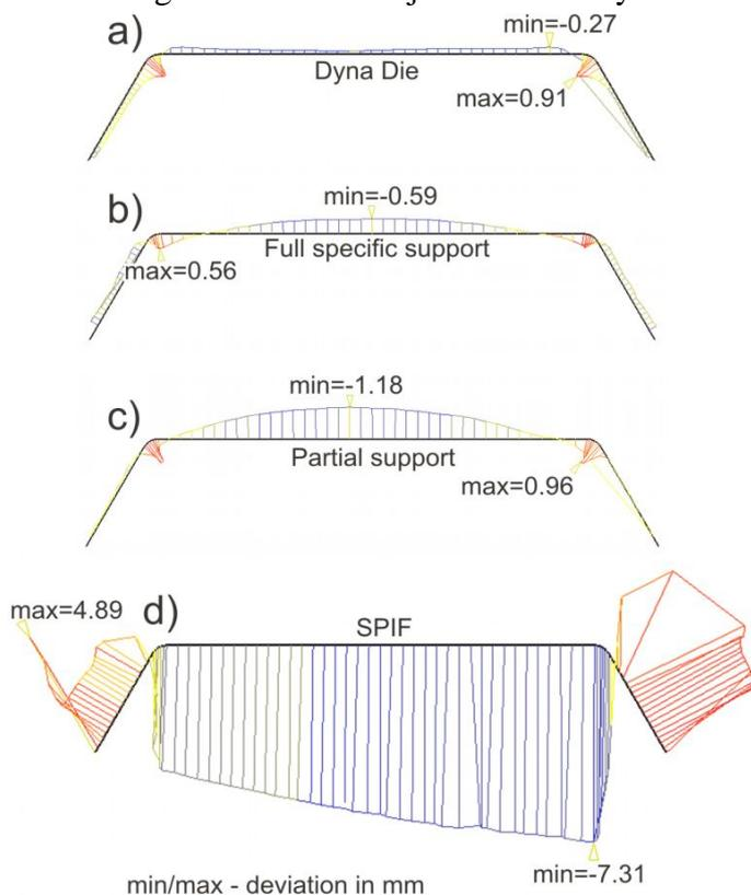
Fig. 4: Comparison of accuracy for different ISF process variants
