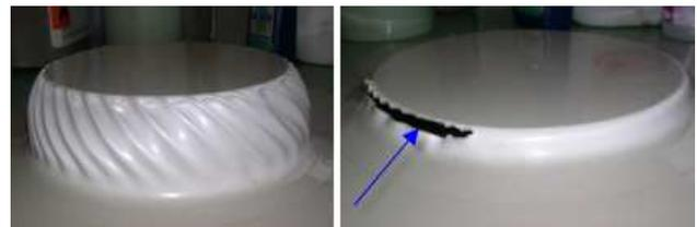
Fig. 3. Mechanical failures on formed part
