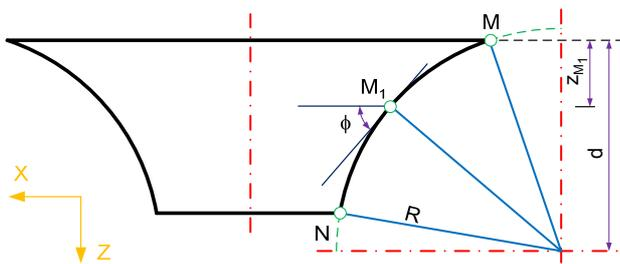
Fig. 1. Geometric illustration of part profile
