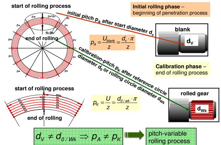
Figure 3: Pitch-specific penetration process into a rolling blank depending upon diameter
