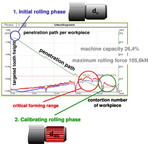
Figure 2: Penetration path into the workpiece
