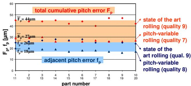
Figure 6: Pitch accuracy with state-of-the-art rolling and pitch-variable rolling (high gear  $m_n=1.6$   $z=10$  - round tools)
