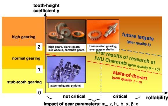
Figure 7: State-of-the-art with gear rolling
