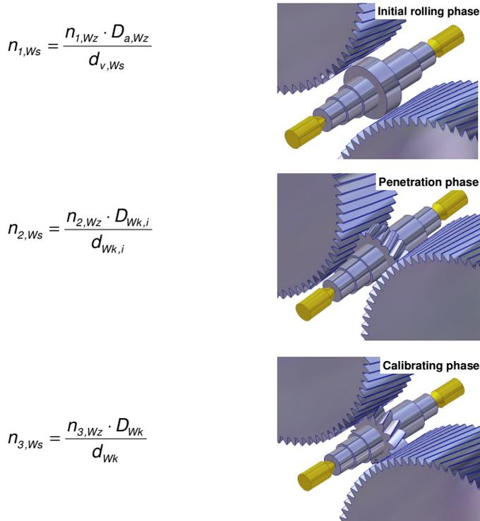
Figure 4: Diameter-dependant speed adjustment in the round rolling process
