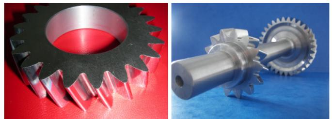
Figure 8: Transmission helical gear rolling into the full material for the first time at IWU (reverse gear at VW AG)
