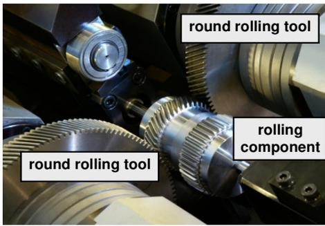
Figure 1: Round rolling technique with two rolling tools
