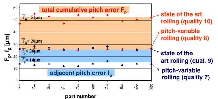
Figure 5: Pitch accuracy with state-of-the-art rolling and pitch-variable rolling (high gear  $m_n=1.6$   $z=10$  - flat tools)
