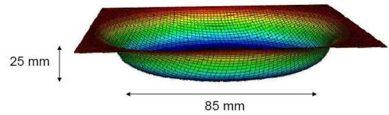
Fig. 3. Final geometry of the cup
