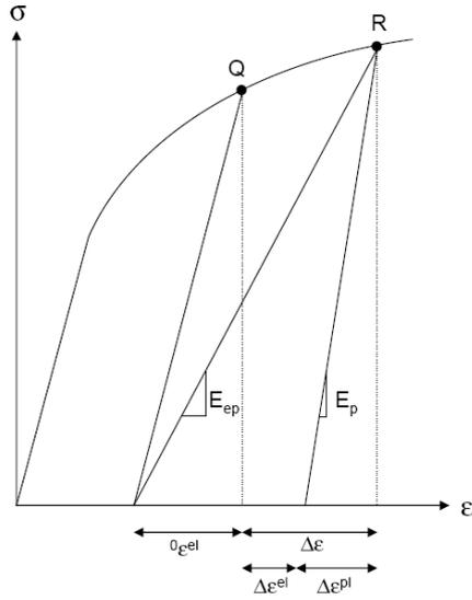
Fig. 2. Incremental deformation method
