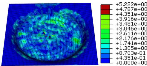
Fig. 6. Equivalent plastic strain error (%)
