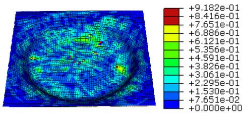
Fig. 5. Stress flow error (%)
