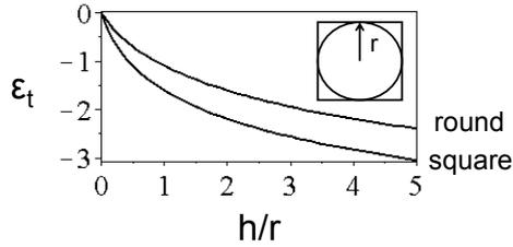
Fig. 1. Thickness strain for different  $h/r$  ratios.
