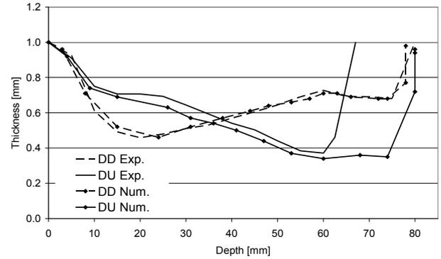
Fig. 4 Comparison of thickness from experiments and simulations as function of depth.
