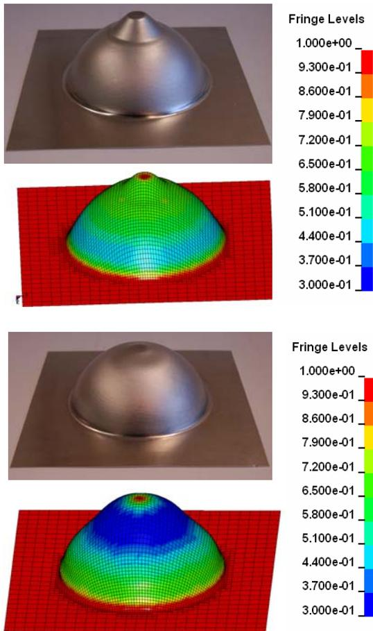
Fig. 3 Comparison of geometry achieved by simulation and by experiment for DD strategy (top) and DU strategy (bottom). Legend displays thickness in mm.
