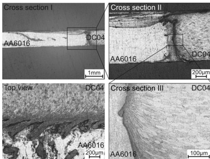
Fig. 4. Appearance of the weld seam in a cross section (I-III) and a top view
