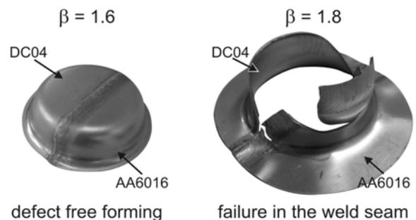
Fig. 3. Results on deep drawing of laser assisted friction stir welded steel aluminium circular blanks
