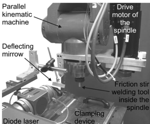
Fig. 1. Setup for laser assisted friction stir welding
