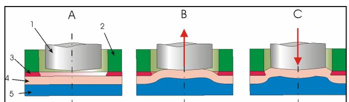
Fig. 2. Operational sequence of the Hydro-Clinching
