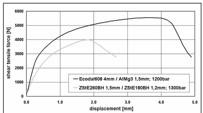
Fig. 6. Shear tensile strength of joints of aluminium and steel sheet metal (Böllhoff self-pierce rivet 35B2, hardness 330 HV10)
