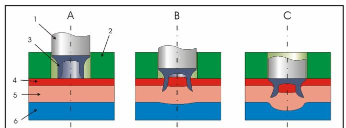
Fig. 1. Operational sequence of the Hydro-Self-Pierce Riveting
