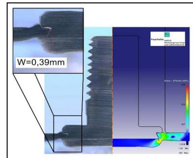
Fig. 9. Comparison between experimental and simulated section of hydro functional element (DC04, 1,5 mm)
