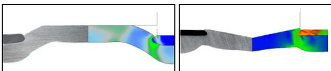
Fig. 8. Comparisons between experimental and simulated sections of hydro clinched sheets. left: joint with stationary and plane punch right: optimized joint with active punch movement and punch front angle of  $160^\circ$
