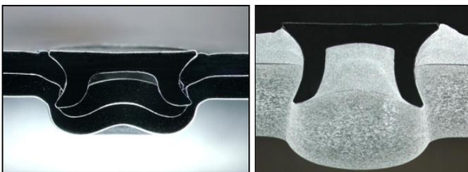
Fig. 5. Polished sections of joints created by Hydro-Self-Pierce Riveting with wobble movement, left: a joint of steel sheets (ZStE180BH 1,2 mm / ZStE260BH 1,5 mm, pressure 1800 bar), right: a joint of aluminium sheets (AlMg3 1,5 mm / Ecodal608 4,0 mm, pressure 1200 bar)
