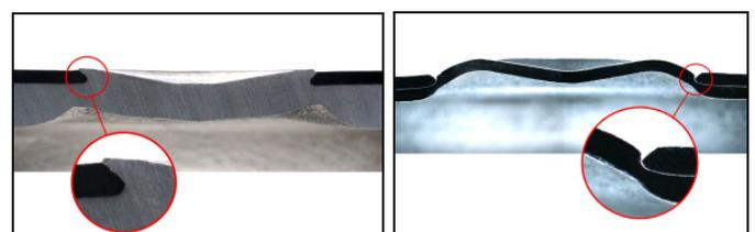
Fig. 7. Cross sections of joints created by Hydro-Clinching with active punch movement; left: DC04 1,0 mm / AlMg0,7Si 4,0 mm; point diameter 17,5 mm; pressure 1600 bar, right: ZStE180BH 1,2 mm / ZStE260BH 1,4 mm; point diameter 22,0 mm, pressure 1400 bar
