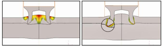
Fig. 4. Damage value distribution at the material separation (left: by Cockroft & Latham; right: by Frobin)
