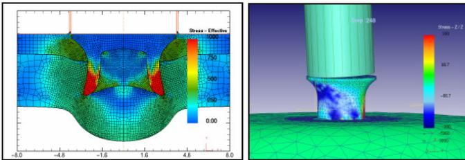
Fig. 3. left: 2D-Effective stress distribution at the end of the joining procedure Hydro-Self-Pierce Riveting, right: 3D-Axial tension distribution during the wobble movement of the punch
