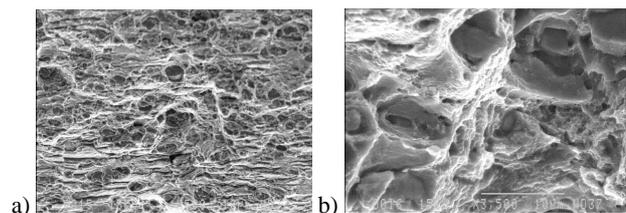
Fig. 4. Fracture surface of a sample specimen with 500x (a) and 3500x (b) magnifications
