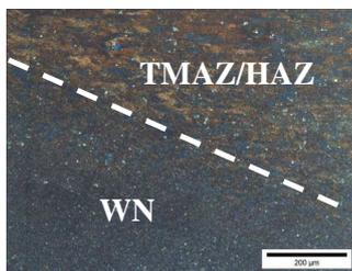
Fig. 2. Microstructure and boundary between the different zones of a sample weld from configuration number 1
