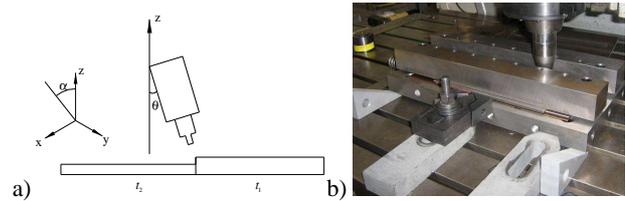
Fig. 1. A schematic drawing (a) and a picture (b) of the weld setup illustrating the inclination and tool angles
