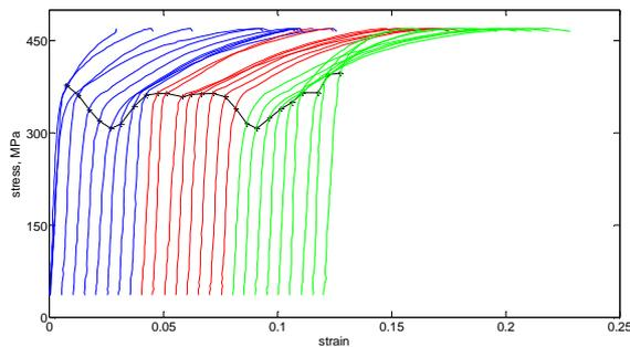
Fig. 7. The local stress-strain curves and the yield strengths from the advancing to the retreating sides of a sample weld
