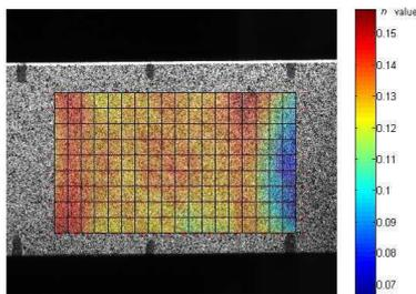
Fig. 6. Local values of the strain hardening exponent around the weld centreline
