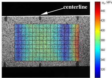
Fig. 5. Local yield strength values around the weld centreline
