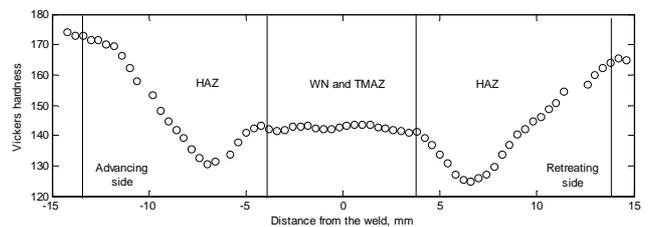
Fig. 3. Hardness profile of a weld from configuration number 1
