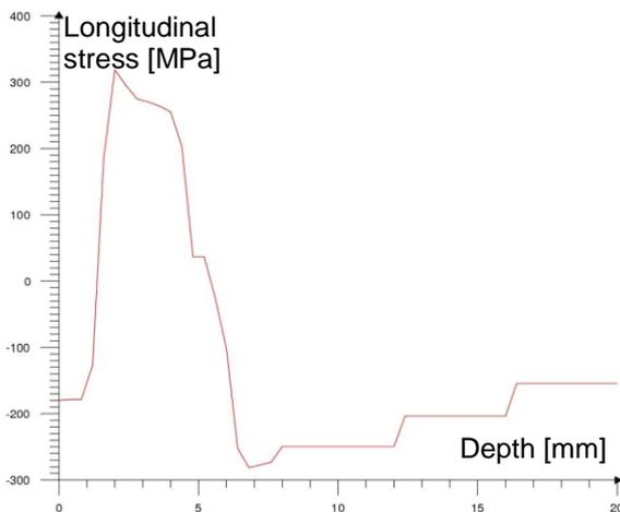
Fig. 7. Distribution of the residual longitudinal stress with metallurgy ( $v=50 \text{ mm.s}^{-1}$ )
