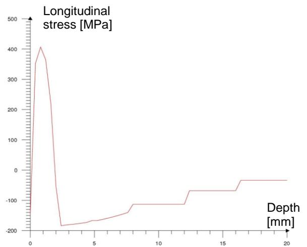
Fig. 6. Distribution of the residual longitudinal stress with metallurgy ( $v=150 \text{ mm}\cdot\text{s}^{-1}$ )
