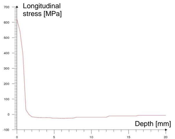
Fig. 5. Distribution of the residual longitudinal stress without metallurgy
