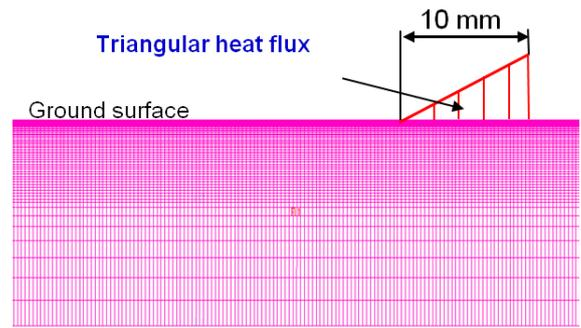
Fig. 2. Mesh and model load.
