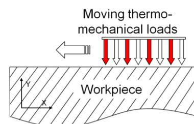
Fig. 1. The global model of grinding
