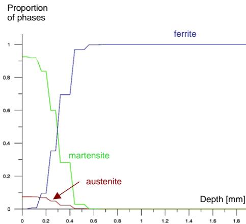
Fig. 4. Simulated proportion of phases.
