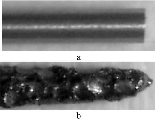
Fig. 4. - Electrode tool: a) ET before machining; b) electrode tool wear after machining process at upper values of voltage, capacity and liquid density
