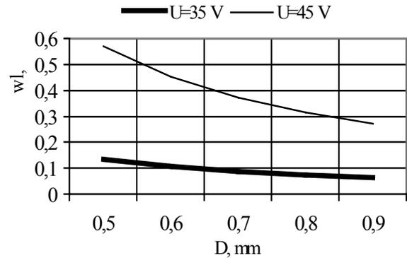
Fig. 2. Influence of electrode tool diameter on electrode tool axial wear
