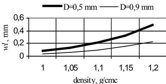
Fig. 6. Influence of the work liquid density on the electrode tool wear
