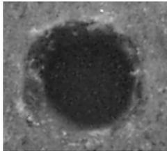
Fig. 5. Hole obtained by ECDM in a cutting steel workpiece
