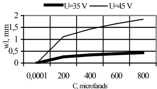
Fig. 3. Influence of electric capacity on electrode tool axial wear
