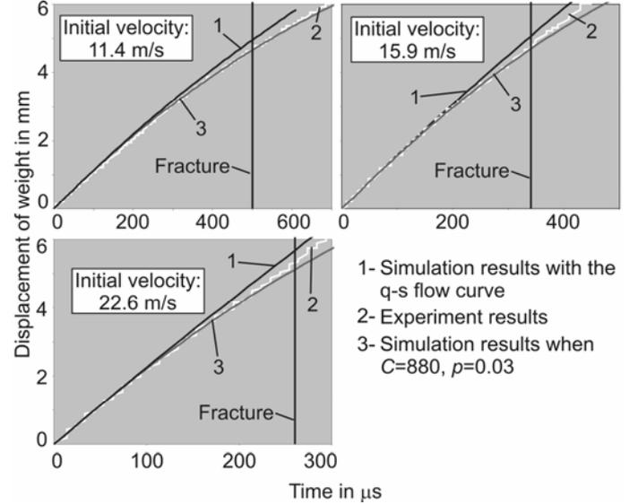
Fig. 4 Measured and calculated plunger displacement courses
