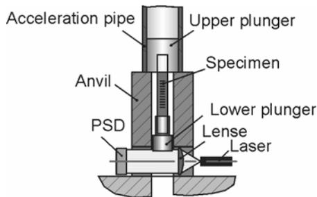
Fig. 2 Principle of Laser-PSD
