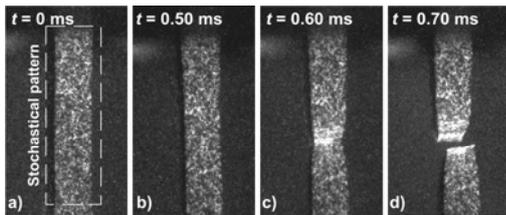
Fig. 6 Photos from a high speed tensile test. a) initial state, b) elongation, c) fracture, and d) the state after the fracture
