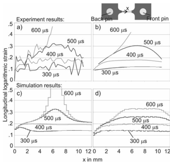
Fig. 7 Strain distribution courses. a) experiment results, b) trendlines of experiment results, c) simulation results ( $C=p=0$ ), d) simulation results ( $C=880, p=0.03$ )
