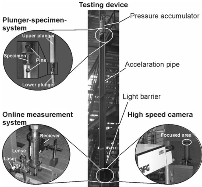
Fig. 1 Experimental setup and measurement systems
