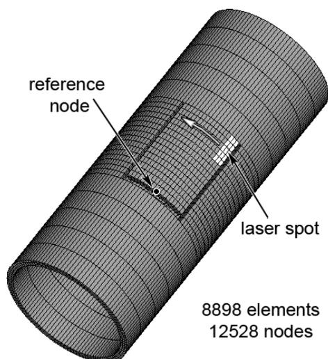
Fig. 1. FEM model for laser forming
