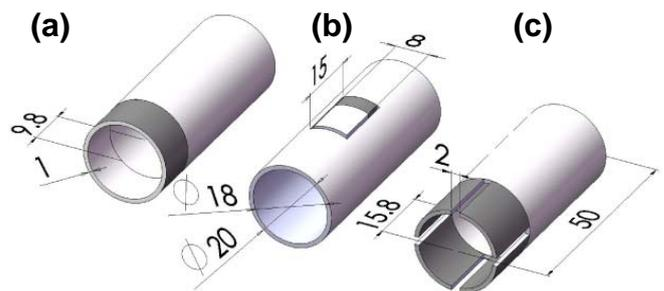
Fig. 2. Samples for laser forming tests
