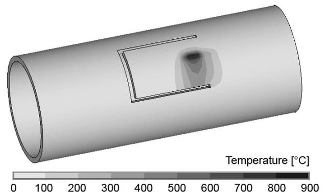
Fig. 5: Temperature map after 1 s (point 2).
