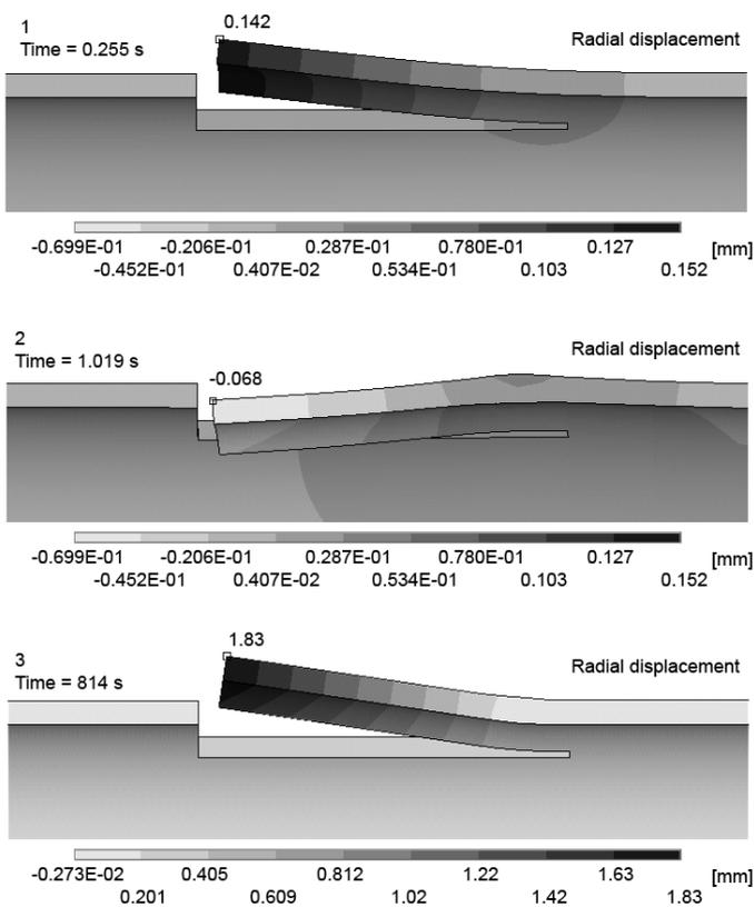
Fig. 6: Radial displacement maps (section view) at three different time steps.
