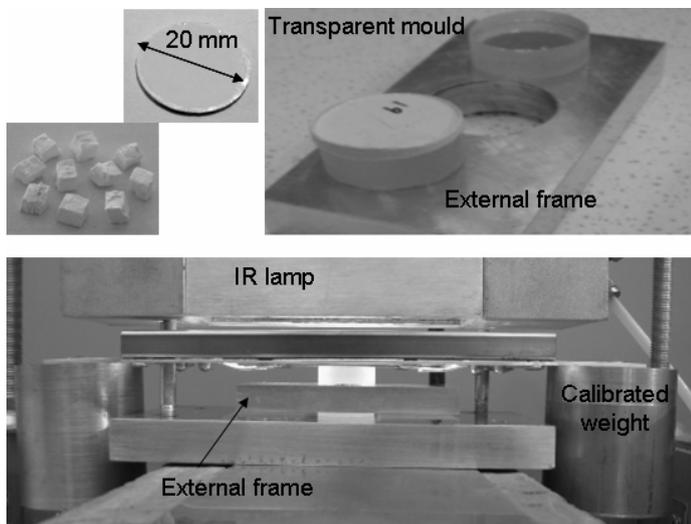
Fig. 1. Experimental apparatus for direct pellet moulding.
