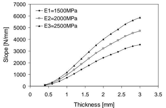
Fig. 4. Plate bending simulation: numerical slope as a function of the disk thickness for different elastic modulus.
