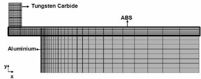
Fig. 3. 2D mesh for the simulation of the plate bending test.
