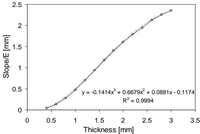
Fig. 5. Plate bending simulation: normalization of the numerical slope as a function of the disk thickness.
