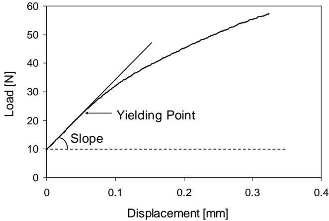
Fig. 2. Plate bending curve for the disk n°7 (moulding phase: 1800 W, 40 s; pre-heating: 1000 W, 40 s).
