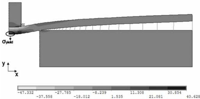
Fig. 6. Simulation of a plate bending test for the disk n°7 (moulding phase: 1800 W, 40 s; pre-heating: 1000 W, 40 s).
