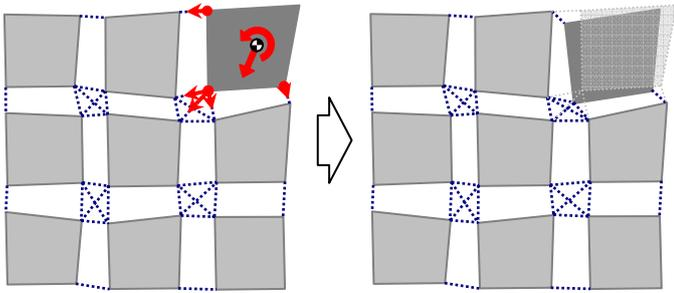
Fig.5. Iterative movement of plane patches by an imaginary spring model
