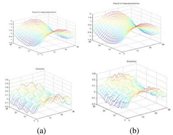
Fig.8. Result of measurement with saddle shape (a) 16 patches (b) 64 patches
