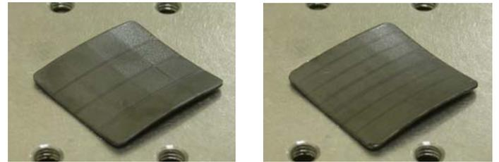
Fig.7. Experimental result of saddle shape (a) 16 patches (b) 64 patches
