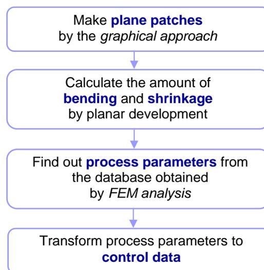
Fig. 1. Overall procedure of 3D laser forming
