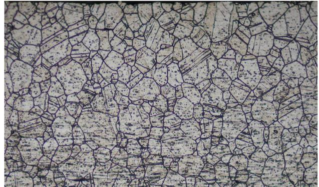
Fig. 6 Annealing twins in laser bending structure, laser power 200 W, speed 8 mm/s, 6 steps, magnitude of 200:1
