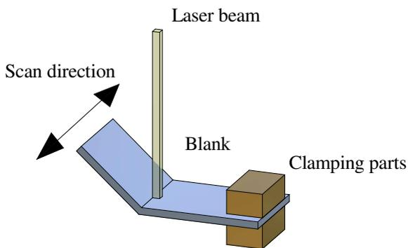
Fig. 1. Schematic view of laser bending
