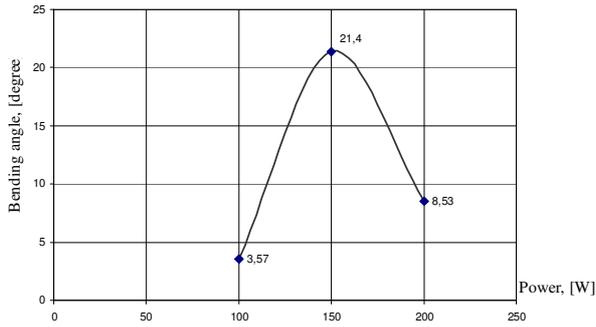
Fig. 2. Bending angle variation for different laser powers, speed 8 mm/s, 6 steps
