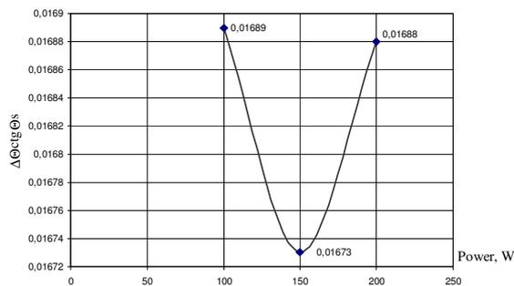
Fig. 4. The first order inner tensions variation for different laser powers, speed 8 mm/s, 6 steps
