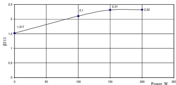
Fig. 5. The second order inner tensions variation for different laser powers, speed 8 mm/s, 6 steps
