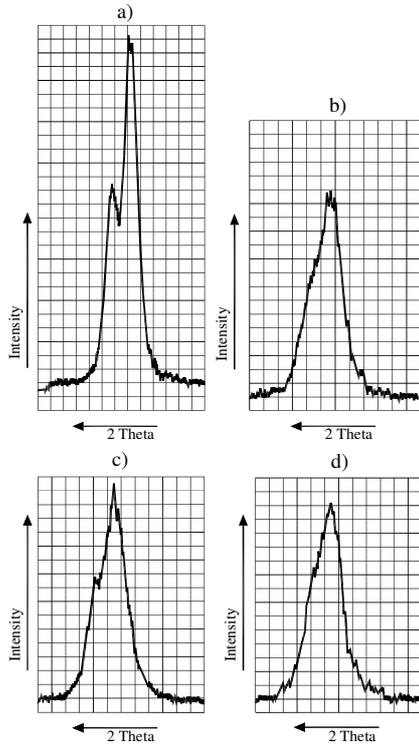
Fig. 3. X-ray diffractogram of the laser machined AISI 304, speed 8 mm/s, 6 steps: a. initial state; b. 100 W laser power; c. 150W laser power; d. 200W laser power (arbitrary units)
