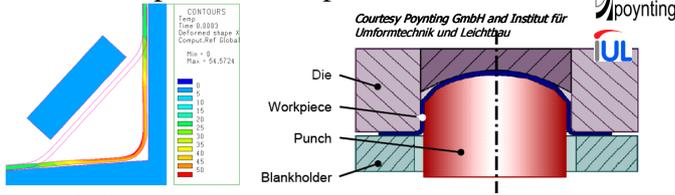
Figure 2: Process description, preformed shape and final shape with temperature field
