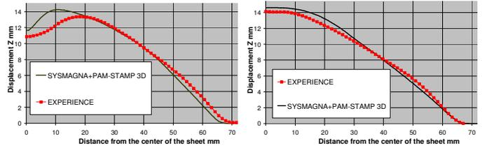
Figure 4: Displacements at the end of the process along the major axis for two charging energies.
