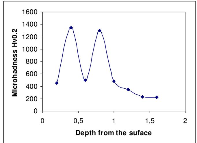
Fig.4. Microhardness measurement of laser clad samples
