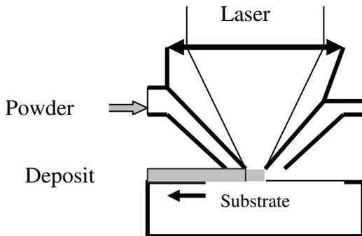
Fig.1. Schematic illustration of laser coating process
