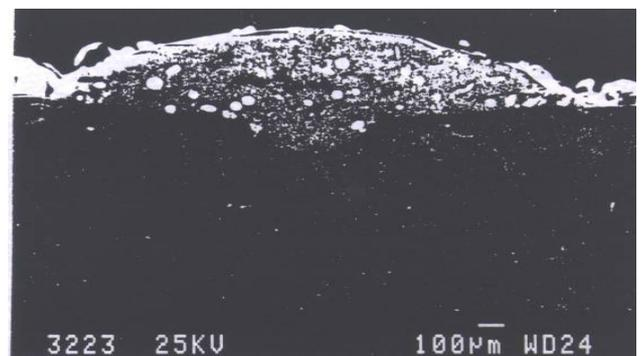
Fig.2. Typical laser clad material: distribution of the spherical tungsten carbides.
