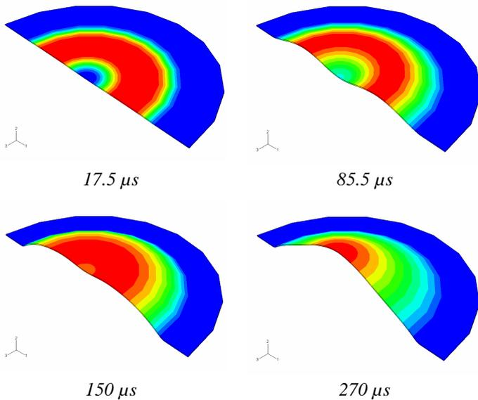
Fig. 4. ABAQUS/Explicit predictions of deformed sheet
