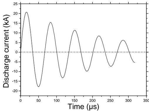
Fig. 1. Evolution of the intensity of the discharge current
