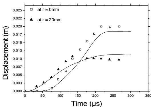
Fig. 5. Vertical deflection U2 of the sheet at radii 0 mm and 20 mm as function of time
