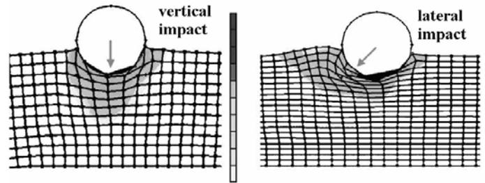
Figure 4. Finite Element Method (FEM) analyze of the impacts: vertical impact (left side) and lateral impact (right side).
