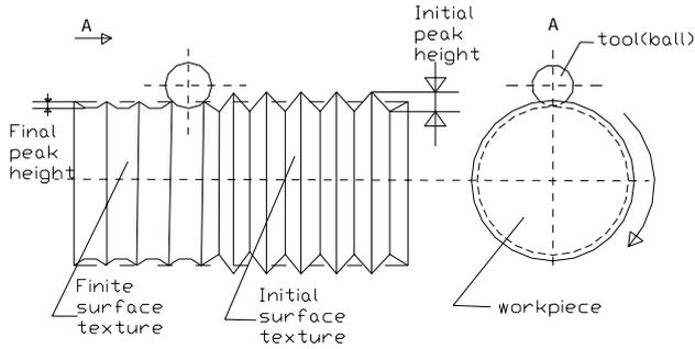
Figure 2. Shape schematization of micro profile.
