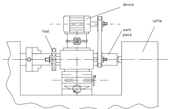
Figure 1. The cold plastic superficial deformation the device scheme.
