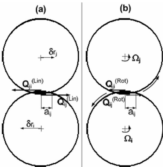
Figure 3. Spheres at elastic impact. a) different rotation value; b) same rotation value.
