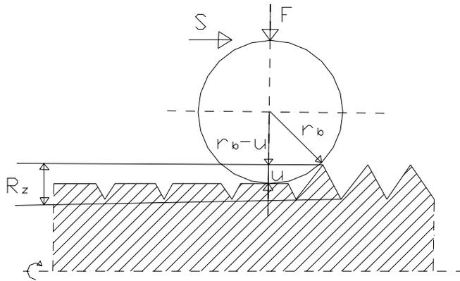
Figure 5. Geometric process model.
