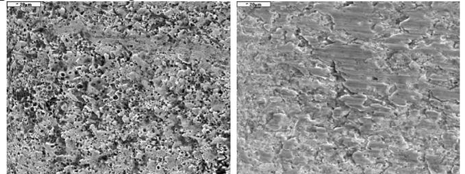
Fig.5. Analyse SEM of contactor: virgin (left), after six tests (right)
