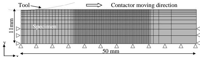
Fig. 3. Numerical model of the upsetting sliding test
