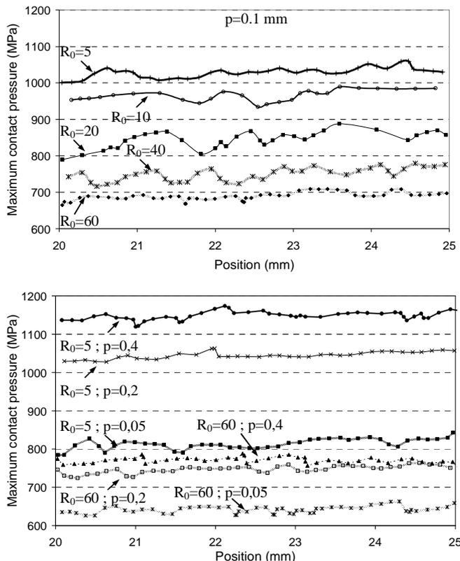
Fig. 4. Influence of parameters ( $p$  and  $R_0$ ) on the maximum contact pressure
