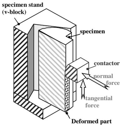
Fig. 1. Design of upsetting sliding test
