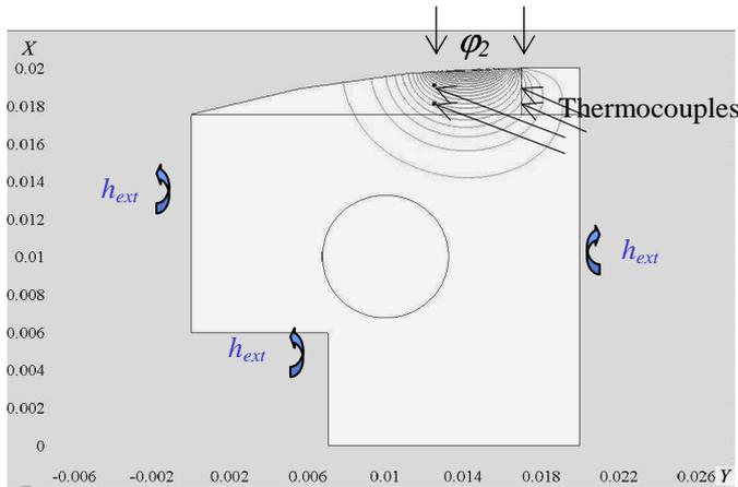
Fig. 4. Measurement principle on tool sub-domain.
