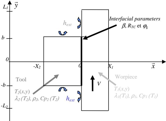
Figure. 1. Global heat transfer model.
