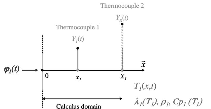
Fig. 3. Measurement principle on workpiece sub-domain.
