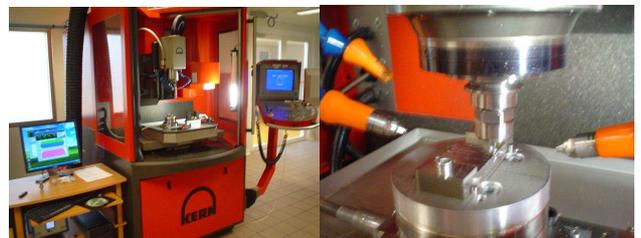
Fig. 3. Experimental data acquisition system used in milling
